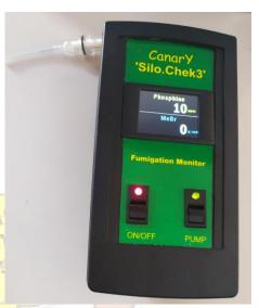
SILO•CHEK 3 Phosphine Monitor is proudly designed and built in Australia to detect & accurately measure the chemical
