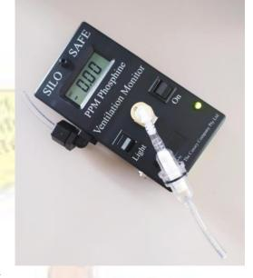
SILO•SAFE-V Phosphine Clearance Monitor is designed and built proudly in Australia to detect low trace levels of phosphine (PH<sub>3</sub>) that may become trapped inside a container following fumigation & ventilation of the stored commodity. A
