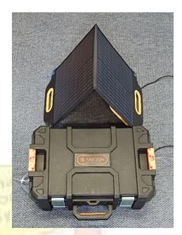
Cloud Canary is designed for use around remote sealed storage containers where real-time fumigant concentration data must be recorded (C/T) and stored for later downloading. Gas samples are pulled from three separate positions in a container of commodity requiring fumigation at a bio-security border control point.
